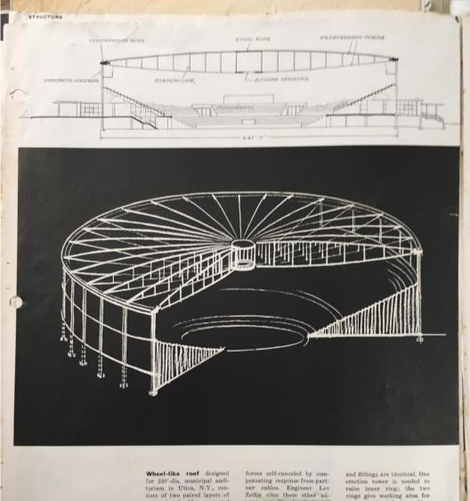
Wheel-like roof designed for 240°-dia, municipal auditorium in Utica, N.Y., consists of two paired layers of pretensioned cables, separated by vertical studs. The 72 cables of each layer are anchored to the inner steel tension ring and outer reinforced eonerete ring which, being under constant compression, needs no expansion joint. Flutter is eliminated and unsymmetrical or upward
