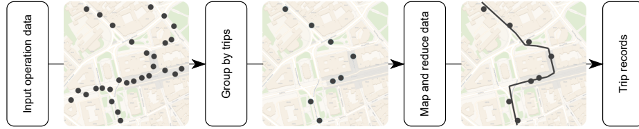
Fig. 3. Three main steps of the transformation algorithm for integrating and compression of real operation big data into the proposed data model. Organizing and storing raw real operations data based on the trips to which that data belongs allows compression, but also preserves all of its external relationships.
